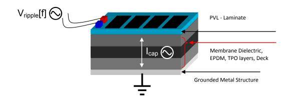
While this does not represent a safety risk, system performance may be reduced if *UNI-SOLAR* PVL laminates are combined with transformer-less inverters.
