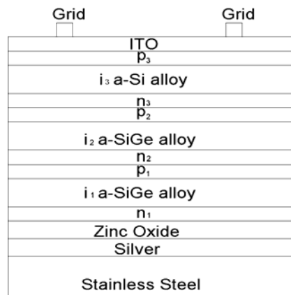
Figure 1. Schematic of triple-junction cell.
